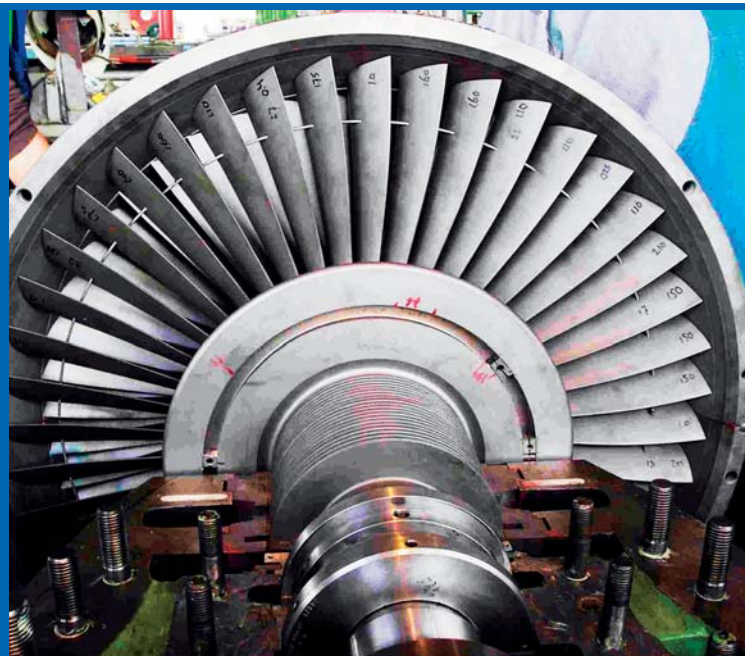
Assembly overview exhaust end.
