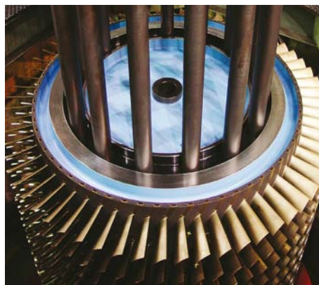
Compressor rotor restack.
