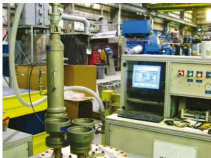
Fuel nozzle flow test.
