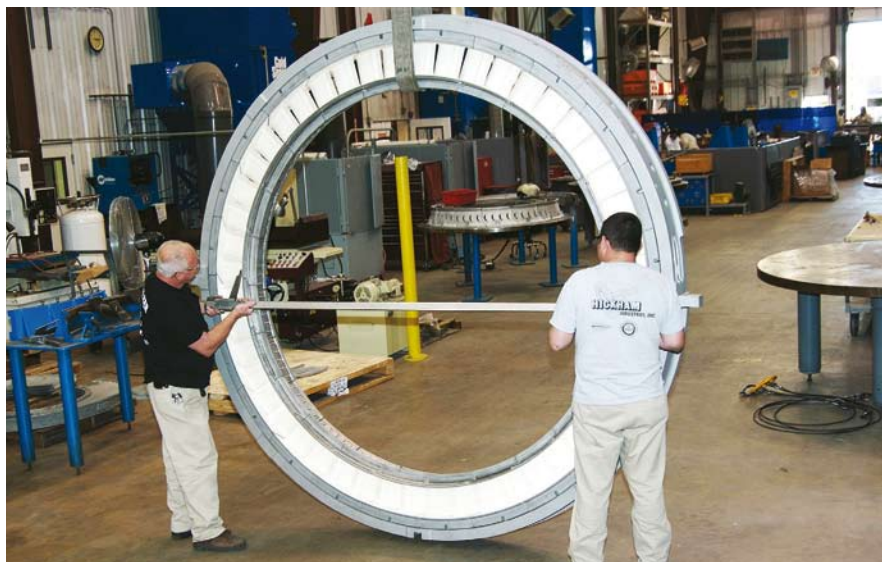
Repaired and coated first stage nozzle.
