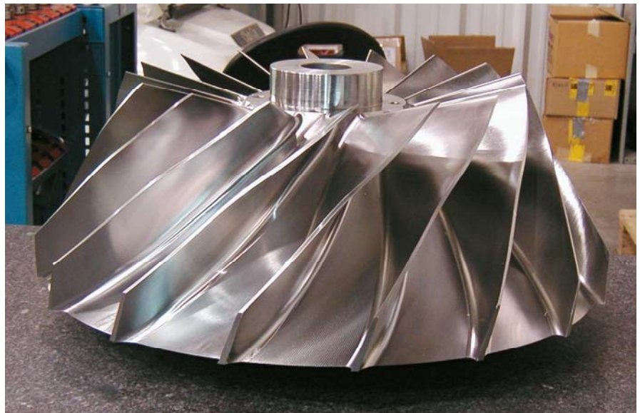
Figure 3 Modern tools allow designing complex blade geometries. Impellers with such new blades have higher capacity and efficiency than older machines with 2D blades.
