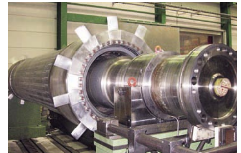
Figure 4: LS-balancing of the rotor.
