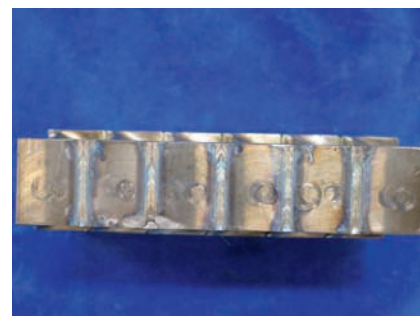
Figure 5: Blade packets after welding.
