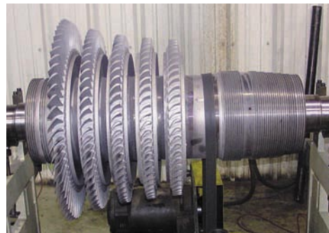
Rotor from wrecked expander.
