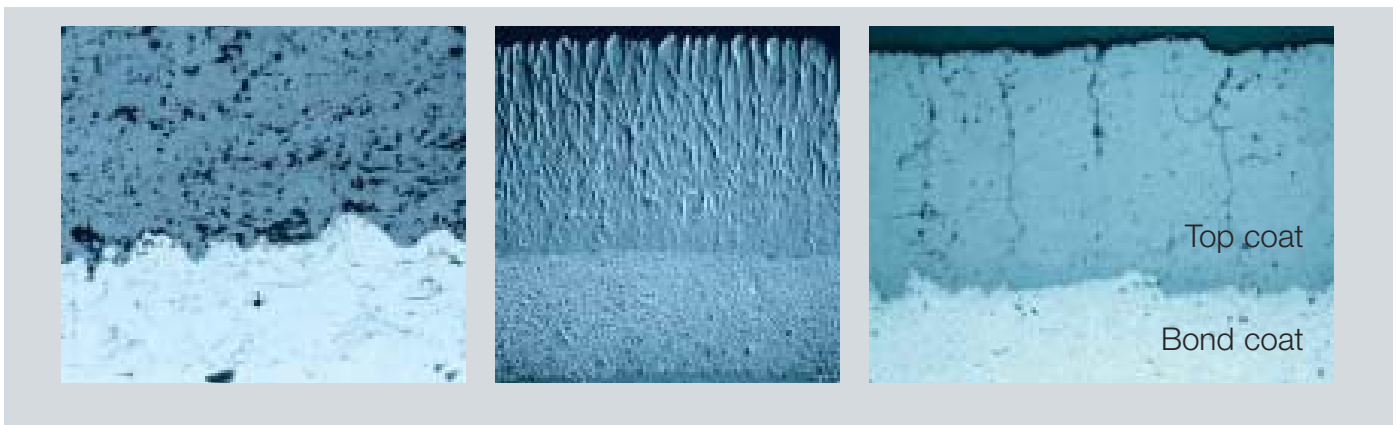
2 Evolution of thermal-barrier coatings (from the left): air plasma spray, EB-PVD, and vertical macro-cracked TBCs.
