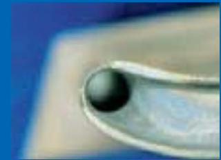
Blade with thin wall section – normal procedure would be to scrap the blade
