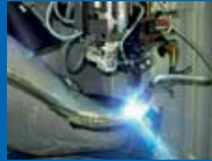
Picture frame being welded to a transition piece
