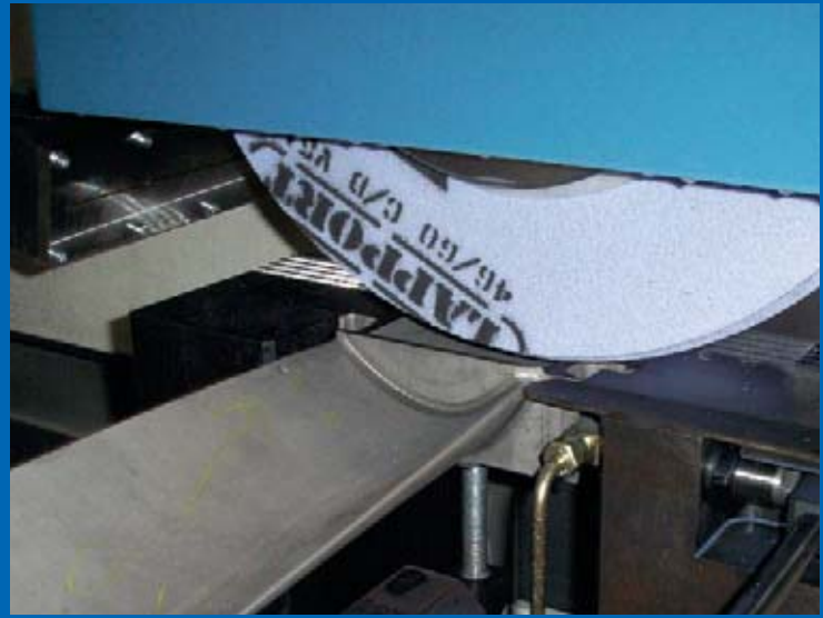
Root grinding 3rd stage blade.
