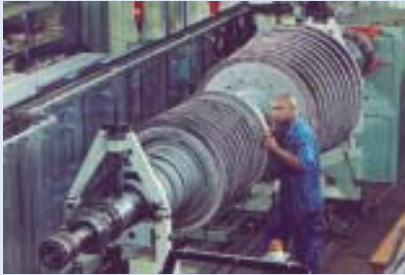
Low balance check of high-pressure steam turbine rotor.
