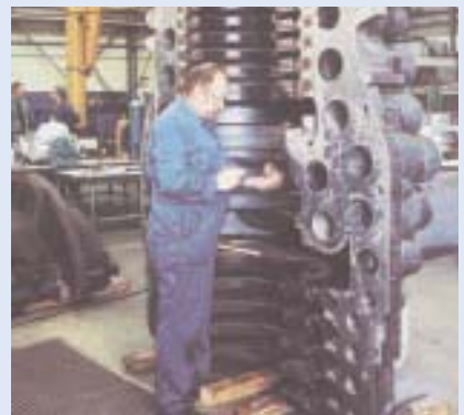
Repair inner casing of steam turbine rotor.
