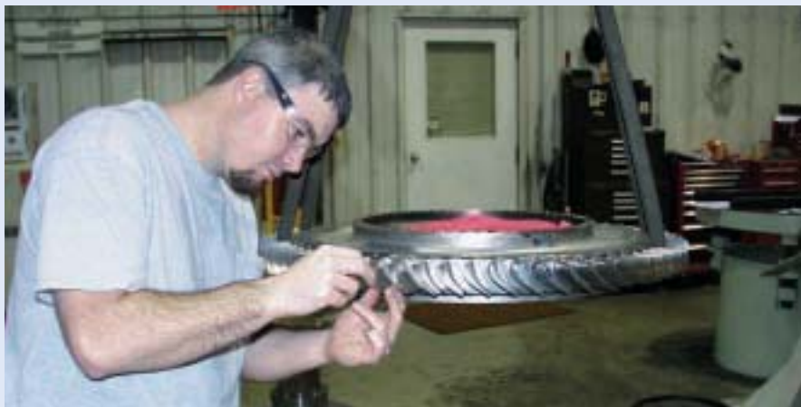
New blades fit-checked in disk.
