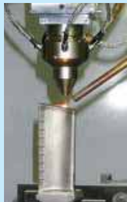
Laser cladding of rotor blades
