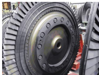
HP rotor of the Frame 3 repaired in our shop
