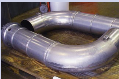
New combustion elbows provided during the course of the job
