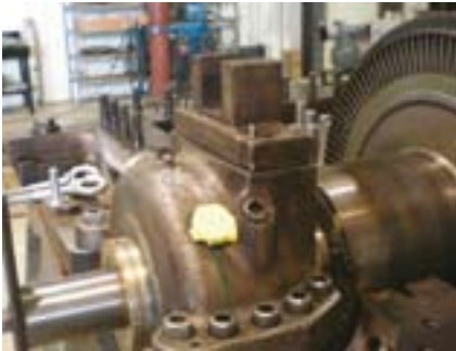
Coupling end bearing housing after re-build.
