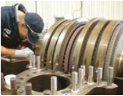
Checking seal clearances during re-assembly.
