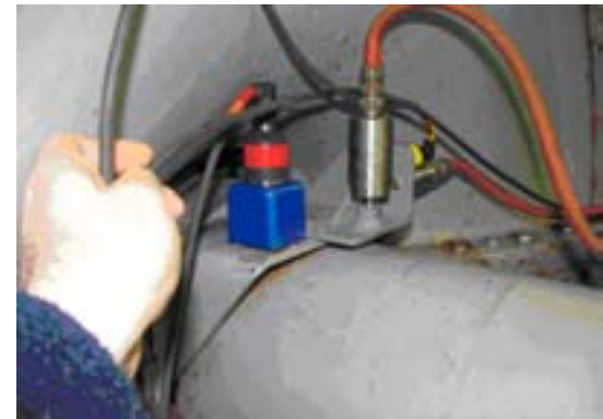
Fig. 4: Velocity transducer bracket on bearing housing
