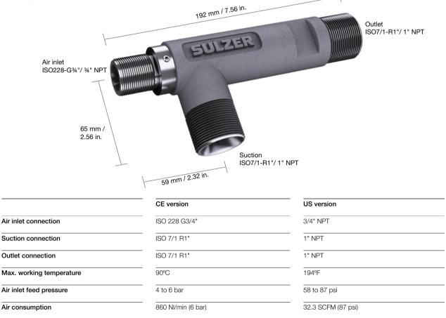
SULZER 716.EJ01 9 412.EJ01 904.EJ01 757.EJ01 Materials Ejector frame (757) ASTM A890 Grade 3A, duplex steel Ejector nozzle (716) ASTM A890 Grade 3A, duplex steel
